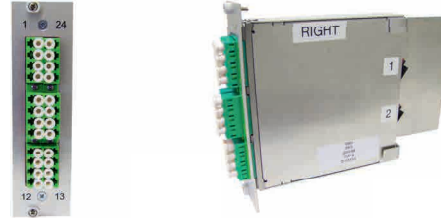
863-10714 | Module compact ½UH, type «B», 1x MPOF (12) LL – 24x LC / APC, SM, OS2
